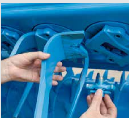
Replacing a quick-change tine
