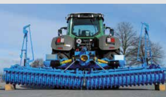
Optimum adjustment to soil by central pendulum axle
