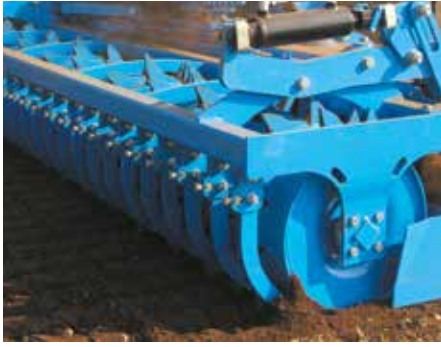
Tooth packer roller for medium and heavy soil conditions
