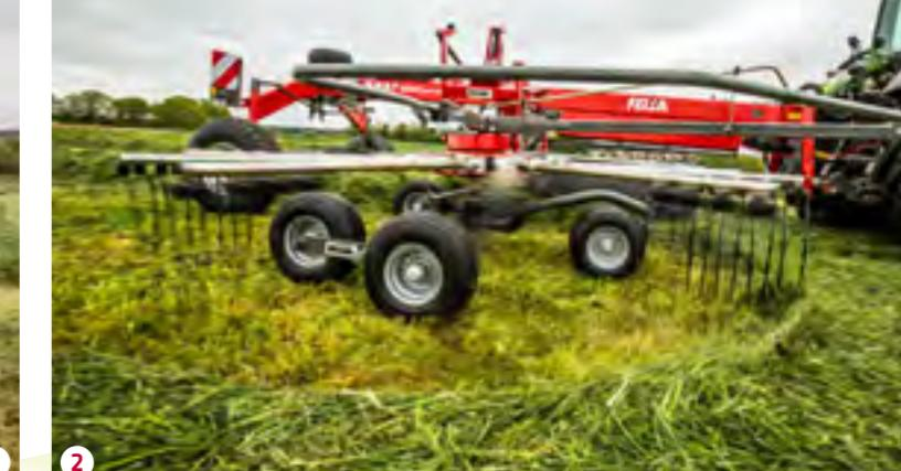
The clearance between the tines and front wheel was also reduced in order to guarantee a top-quality swath without contamination and stones.
