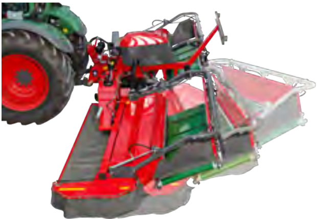
SAFETYSWING approx. 20° to the rear, approx. 620 mm upwards
