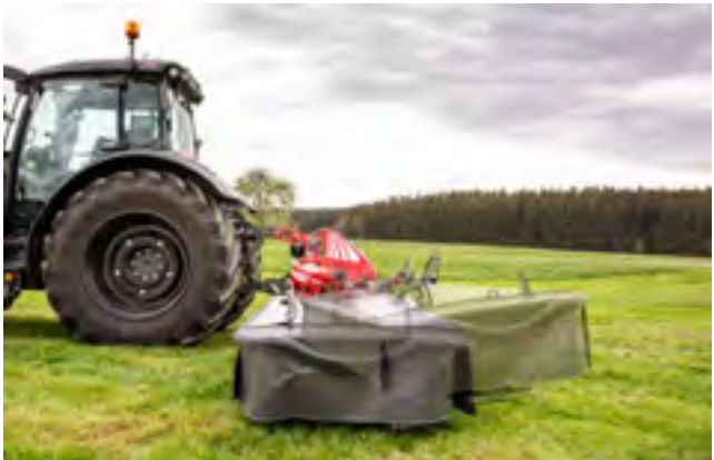
EASYSWING approx. 9° to the rear, approx. 400 mm upwards
