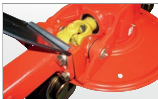
Frame joints that can be relubricated
