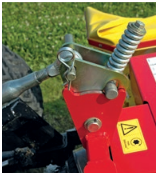
Spring-loaded impact guard (with the FK version)
