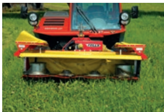
Four mower discs for symmetrically central running
