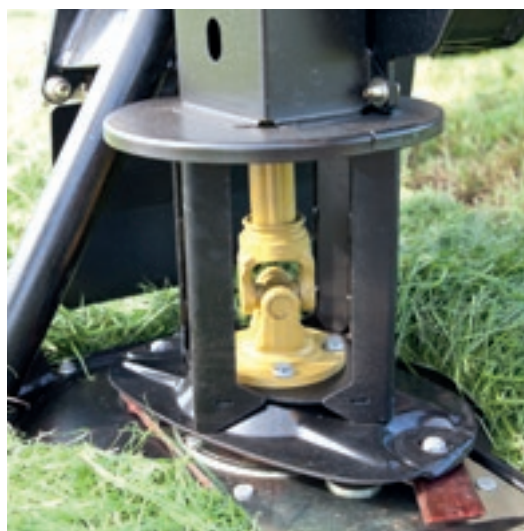
Drive provided from above directly into the first mower
