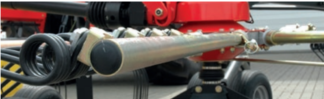
Absolutely smooth front side of the tine arm
