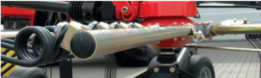
Completely smooth front side of the tine arm
