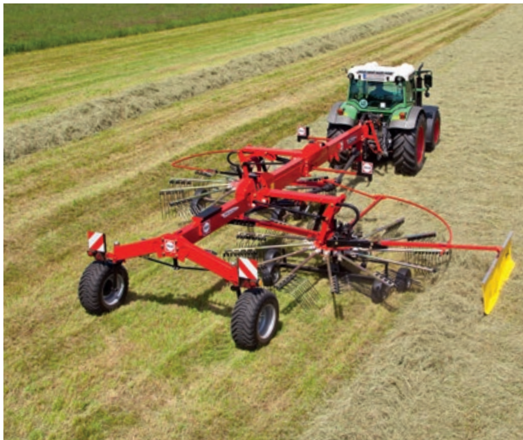
TS 7850 PRO in use (one-swath deposit)
