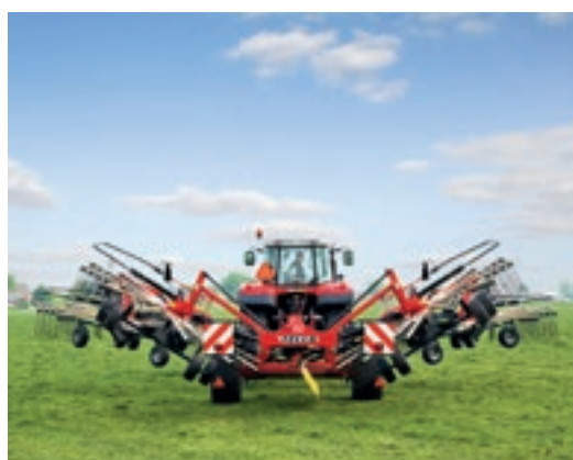
Headland position with automatic height limiter
