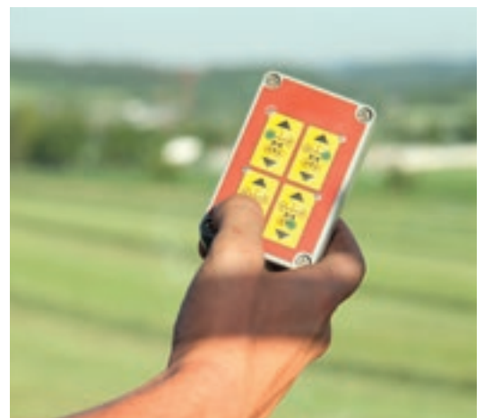
Operating control for electric height adjustment
