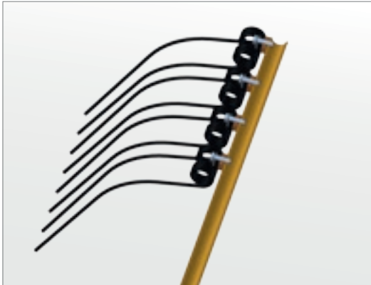
Each tine is bolted in place individually beneath the tine arm
