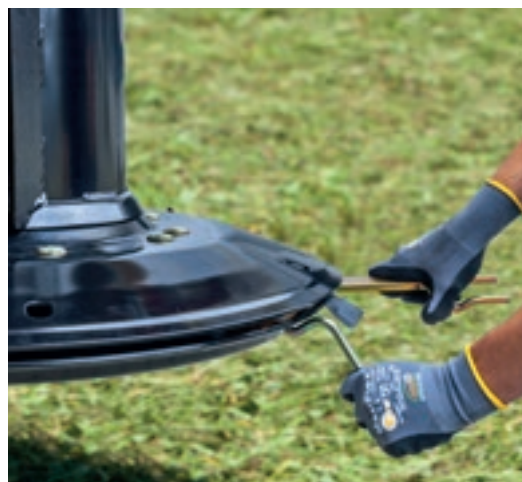
Cutting height adjustment
