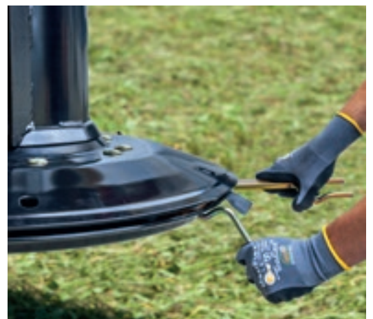
Cutting height adjustment
