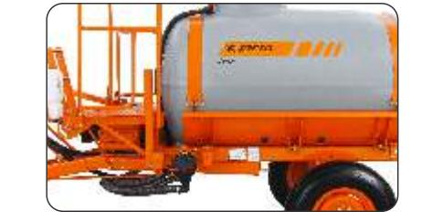
2,000-liter polyethylene corrosion-resistant tank. Sight glass with graduated scale and mechanical agitation system.
