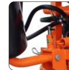
The wings unlock in the presence of obstacles and return automatically to the original position.
