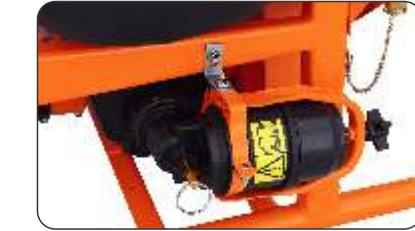
The suction filter retains every type of impurity before it reaches the chemical pump.
