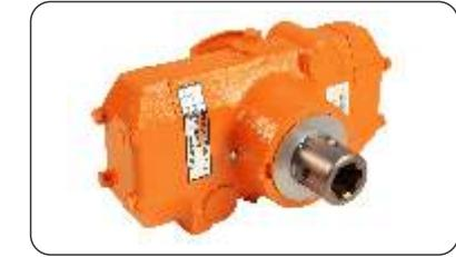
JP-402 pump with two pistons and ceramic sleeves is very resistant to corrosion and abrasion. Flow rate of 38 L/min at 540 rpm. A compensation chamber ensures constant flow rate of the nozzles.
