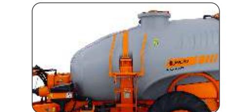
4,000-liter polyethylene and highly resistant to corrosion. Sight glass with graduated scale and mechanical agitation system
