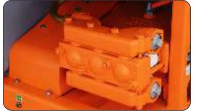
Piston pump with ceramic sleeves is highly resistant to wear. Its sturdiness reduces the number of stops for maintenance and makes the equipment more available for the farmer, thus ensuring application at the correct time.
