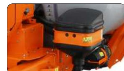
Incorporates the chemical to the tank water thus preparing the mixture in a practical and safe way and reducing risks for the environment and the operator.
