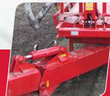
TILTING TOW BAR For easy hook-up to the wrapper
