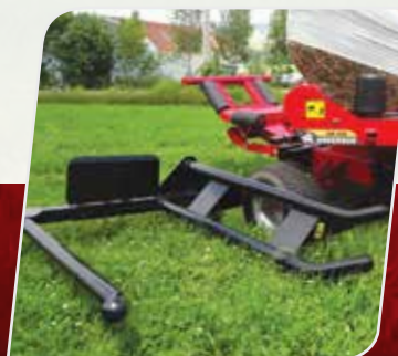
SELF-LOADING ARM Turns bale and loads it onto the wrapper
