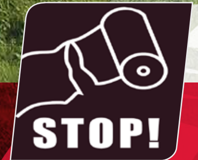
PLASTIC FILM WATCH Automatically stops wrapping process when plastic runs out or tears.
