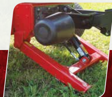
FRONT AND REAR STABILIZER Keep the wrapper level and stable
