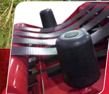
BALE GUIDE ROLLERS Keep the bales centered on the wrapper even when on a slope
