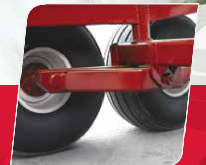
Steerable axle on the trailer
