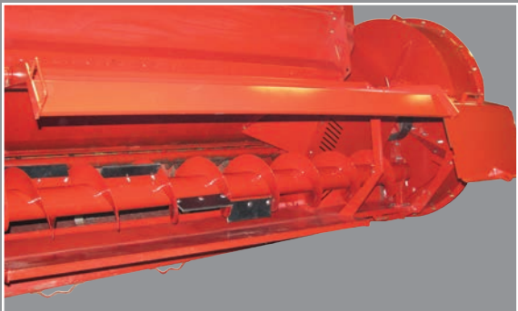
With the door open, the auger paddles hay into a windrow.
