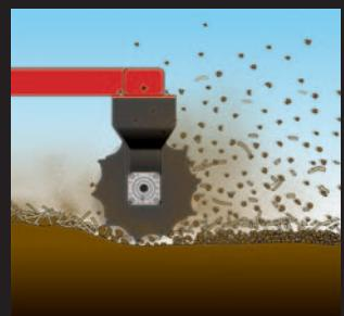
As the Flat bar reel moves forward, the turning action lifts and throws the surface soil out the back for a more level surface. Note: works best behind a disk level'r or disk gang.
