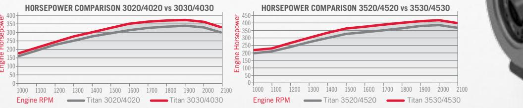
Available in either 330 or 400 HP configurations, the new FPT 8.7-liter engine offers 8-9 percent better horsepower over previous models, with improved efficiency and Tier 4A compliance.
