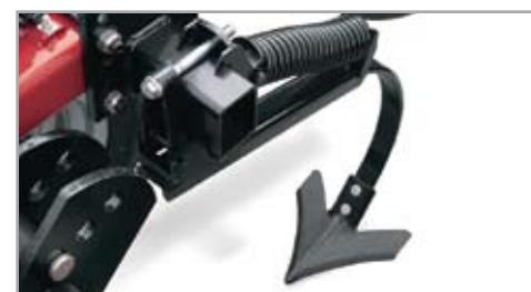
▲ For uniform residue and soil mixing, even in the center between disk gangs, Case IH offers a center shank to remove the uncut soil between disk gangs. The center shank is located farther from the front blades than prior models and has increased holding force.
