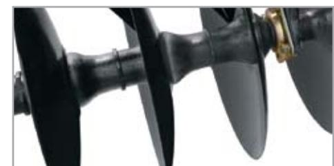
▲ **Earth Metal® blades** feature a crimped-center design for increased blade strength and shallower concavity for better soil penetration with minimized soil compaction. The blades are mounted on nodular cast iron spools for even greater strength and durability.
