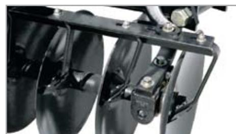
▲ Rigid Arm Scrapers work best in heavy soil, low residue conditions, while Flex Arm Scrapers work in lighter soil or high residue conditions to keep blades free of mud and residue.
