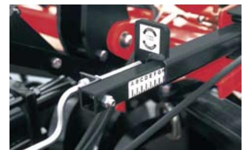
▲ **Single-point, crank-operated hydraulic depth control** is precise and easy to use, and substantially reduces the time required to adjust the depth for various field conditions.
