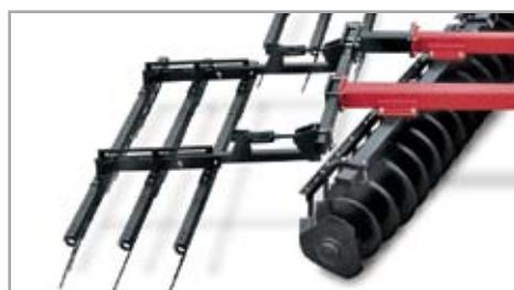
▲ Choose the 3-bar coil-tine harrow, with greater residue capacity and down pressure, for high-residue areas. The 3-bar spike-tooth harrow offers more aggressive clod sizing in tough, dry conditions, and moderate firming of soil (recommended for light-to-moderate residue conditions).
