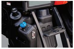
Large Fuel Tank The 34.3 gallon (130 l) fuel tank increases productive work time without the need for frequent re-fueling.
