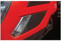
Side Work Lights Standard side lights provide the operator increased visibility when turning.
