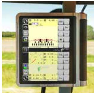
With e-drive II each sowing unit is driven individually via an electric motor. All the data is entered and read by an ISOBUS conform terminal like IsoMatch Tellus PRO or Tellus GO+. The sowing distances are infinitely adjustable on the move. All the sowing units can be switched off individually. This solution saves seeds and money!
