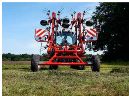
Kverneland 8590 easily converts from transport to working position and fold hydraulically.
