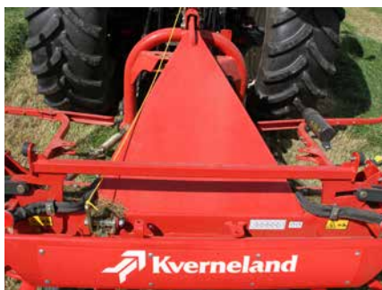
Strong and sturdy mainframe design with V-shaped central unit.
