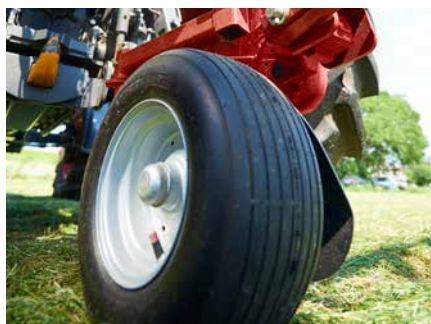
All tedders can be equipped with a third wheel to ensure correct set-up of the tedder independent from tractor and driver.
