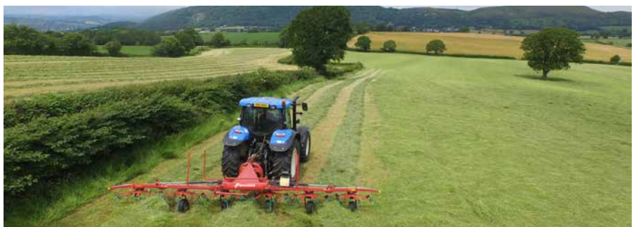
To increase productivity these tedders are equipped with a mechanical border tedding device. Optionally a hydraulic solution is available. A marker shows the position of the axle.
