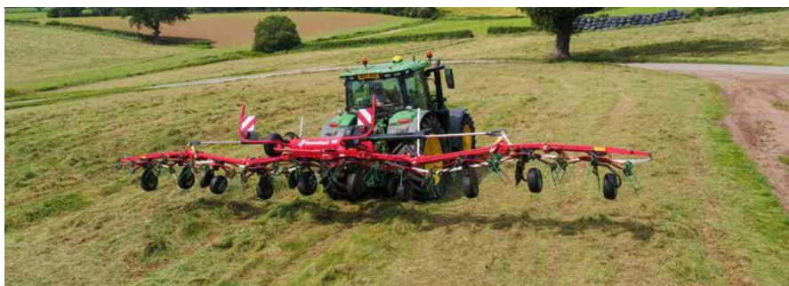
The optional hydraulic headland kit easily stabilises the tedder during headland turning.
