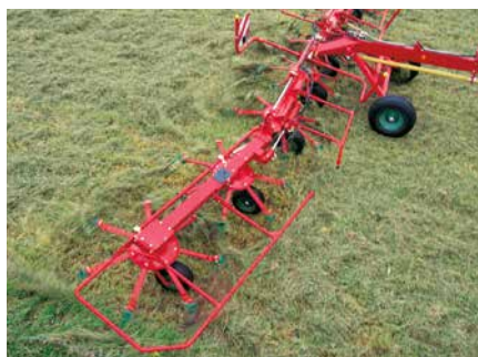
For border tedding the outer rotors are pivoted, to secure evenly inward spreading.
