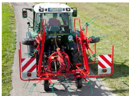
All tedders fold hydraulically from working to transport position and vice versa.
