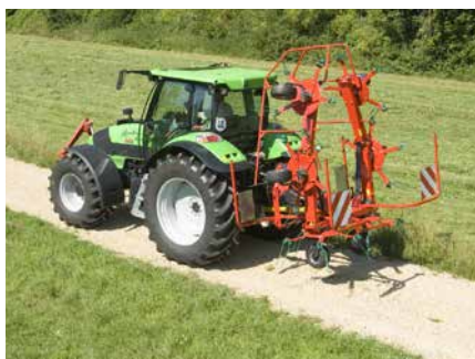
Kverneland 8460 folds hydraulically from working to transport position and vice versa.
