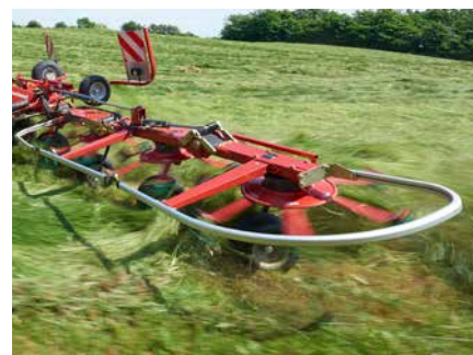
Aluminium rail guards, which are low in weight, but still extremely impact resistant.
