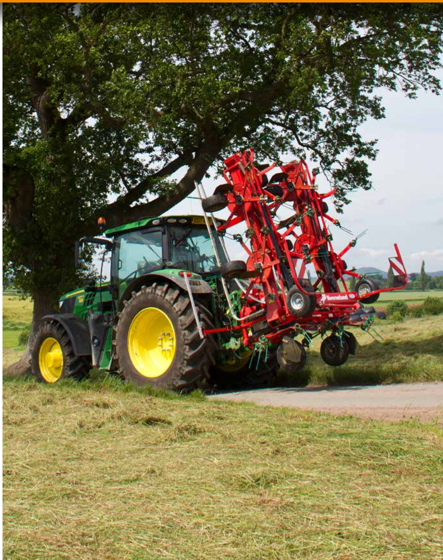
Compact transport dimensions of Kverneland 85112 – storage height is only 3.8m.
