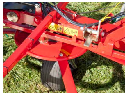
Kverneland 8446 and 8452 are centrally adjusted for border tending.
