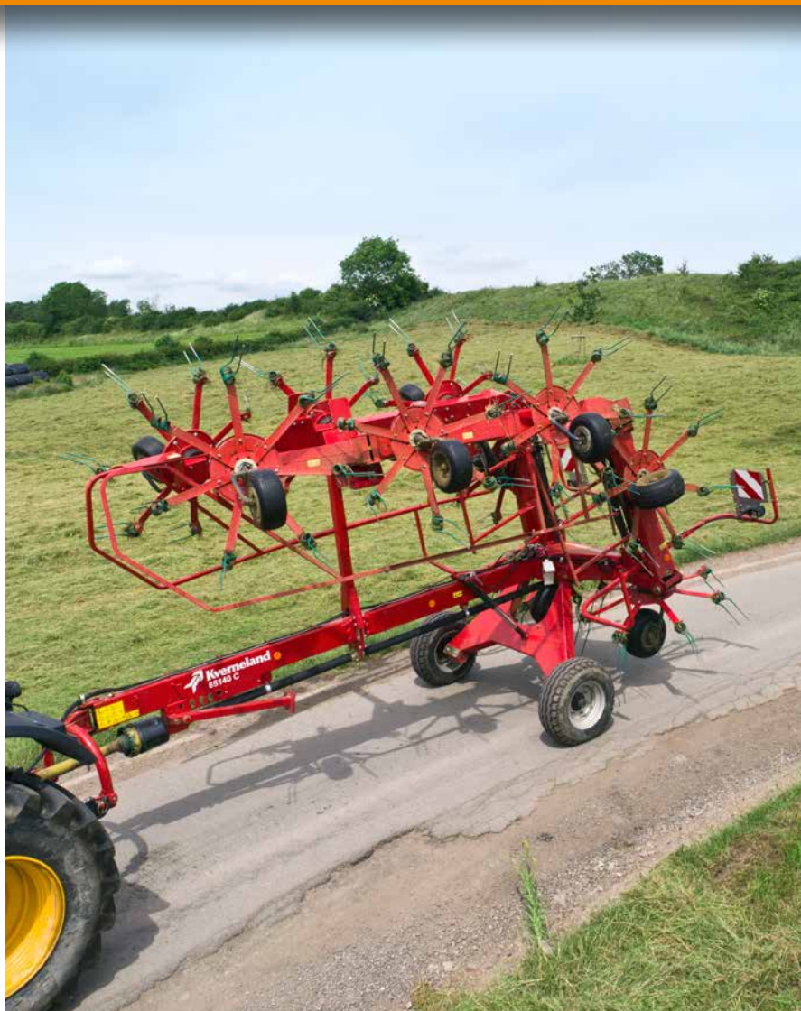
During transport both tedders have a height of only 3.35m and a width below 3.00m.
