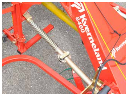
Standard oscillation dampers ensure an even spreading pattern.
