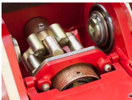
Kverneland HexaLink finger clutch permits the rotors to fold 180° for transport.
