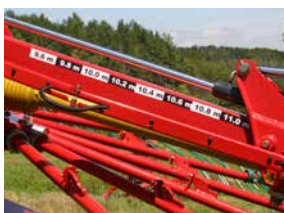
Hydraulic adjustment of working width between 9.60m and 11.00m.
