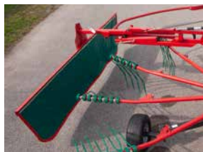
Automatic fold-able swath board with parking stand.
