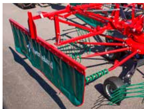
Automatic fold-able swath board with parking stand.
