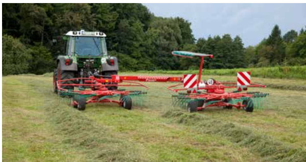
Placing two smaller night swaths.
