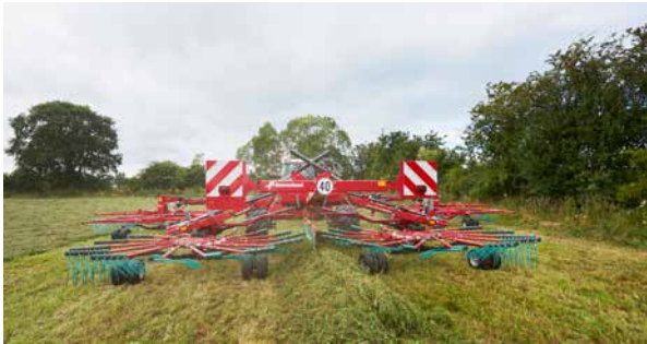
Hydraulic adjustment of swath width.
