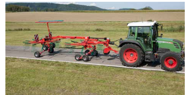
Pulled axle suspension for smooth running characteristics and reduced power requirement.
