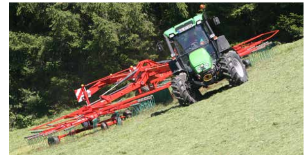
Active wheel steering, allowing sharp turns on headlands and during transport.
