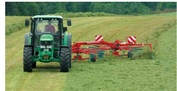
SideShift to the left - raking without driving on unraked crop.
