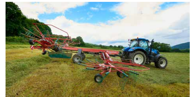
Individual pairwise lift of front and rear rotors. Adjustable time delay for headland position is standard.
