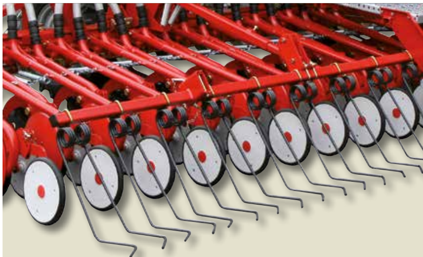
CX-disc couler with wide press wheel (65mm)
