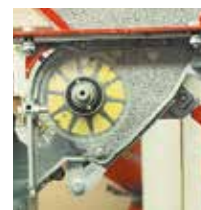
Setting for fine seeds, with rotary brush
