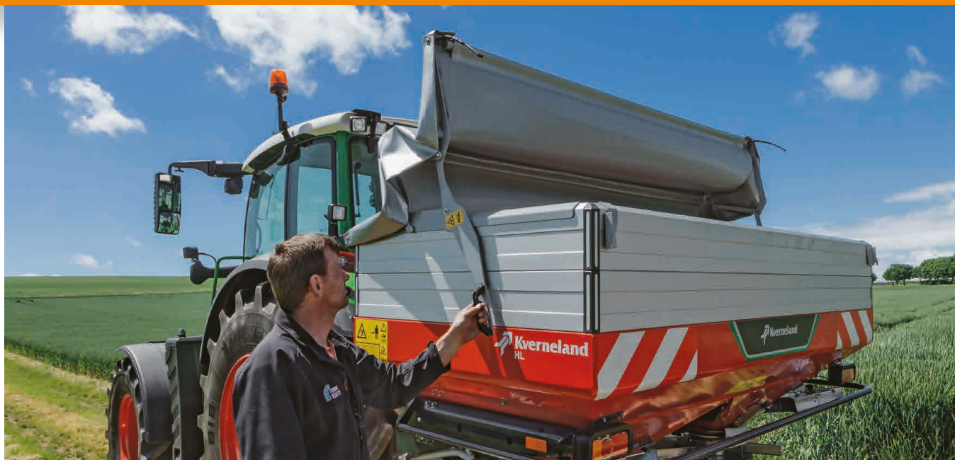
Hopper cover and aluminium hopper extensions
