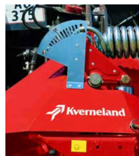
Work smarter on the Go. Hydraulic setting of ground pressure.
