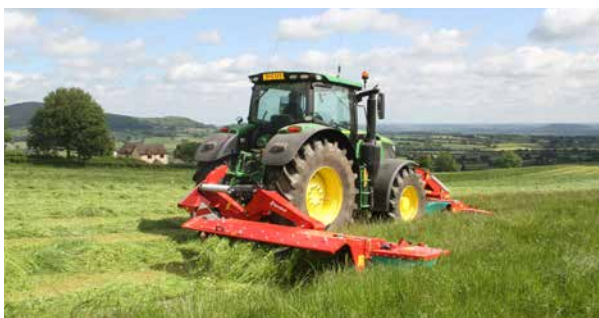
Quick change from swathing to widespreading.
