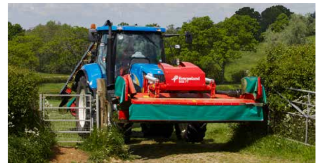
Foldable sideguards ensure narrow transport width.
