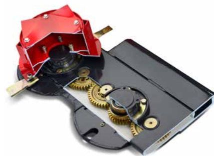
Fully welded cutterbar with overlapping C-profiles for a very strong and stiff construction.
