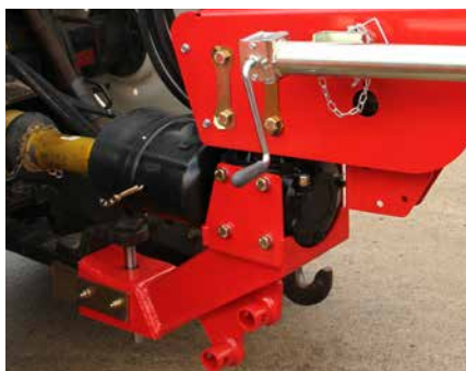
Swivel hitch gearbox with optional clevis connection.
