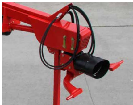
Swivel hitch gearbox with standard 2pt lower linkage connection.
