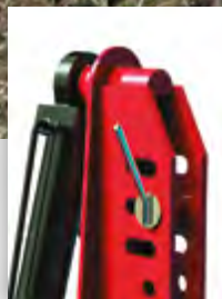
Slotted and inclined top link hole
