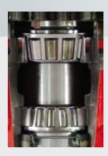
Mounting with double taper rollers
