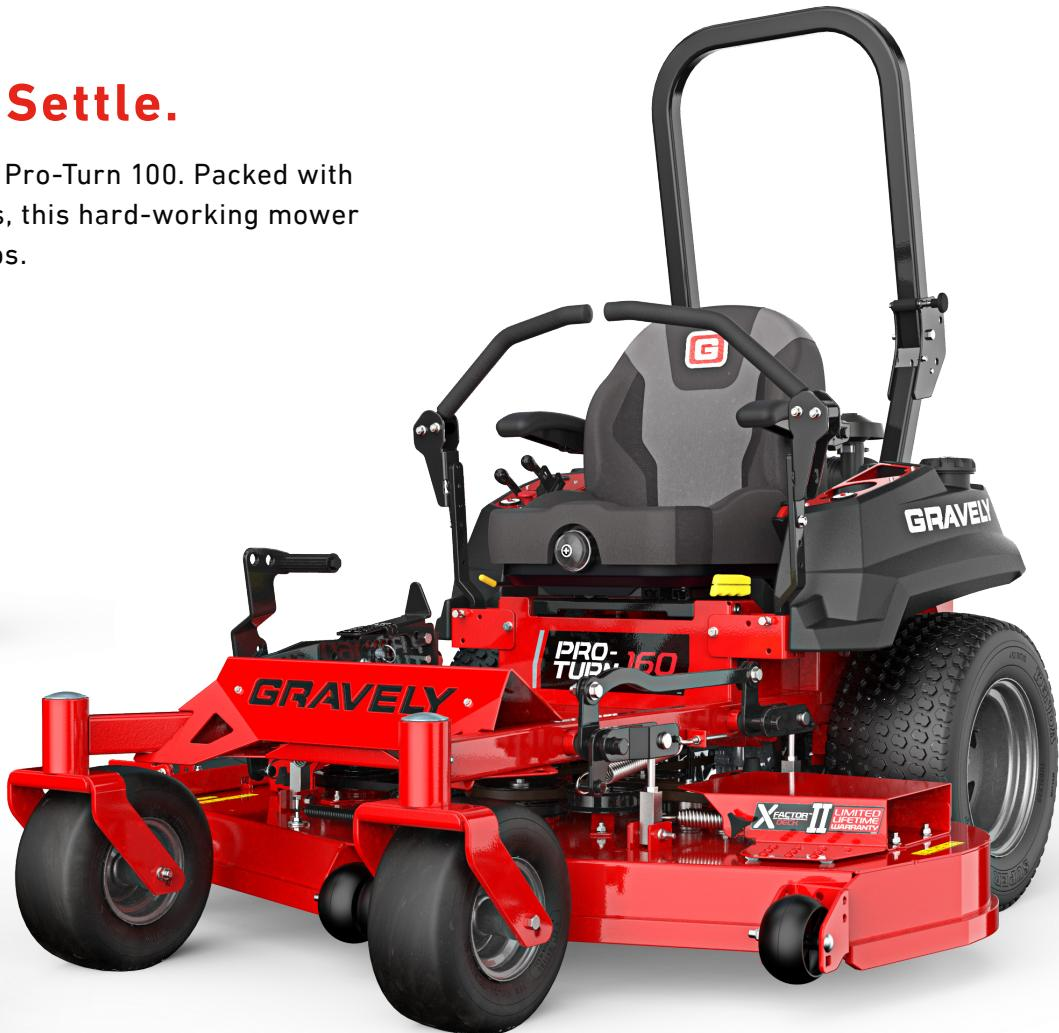
**X-FACTOR® II DECK** The 7-gauge, all-steel welded X-Factor® II Deck is fabricated from top to bottom, providing industrial-strength peace of mind that's reinforced with an exclusive limited lifetime warranty.
