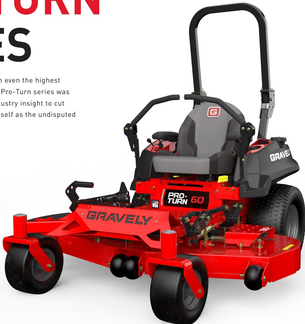
**X-FACTOR® II DECK** is fabricated from top to bottom, providing industrial strength peace of mind.
