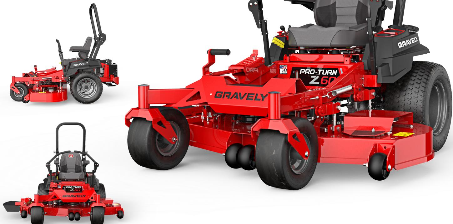
**SEATING SYSTEM** the high-back seat features arm rests, seat isolators and large-diameter steering arms to reduce fatigue and provide all-day comfort.
