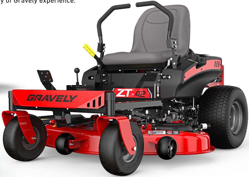
**DECK LIFT** the effortless and intuitive foot-operated deck lift makes it easy to adjust between 7 cutting heights, from 1 1/2 to 4 1/2 inches.
