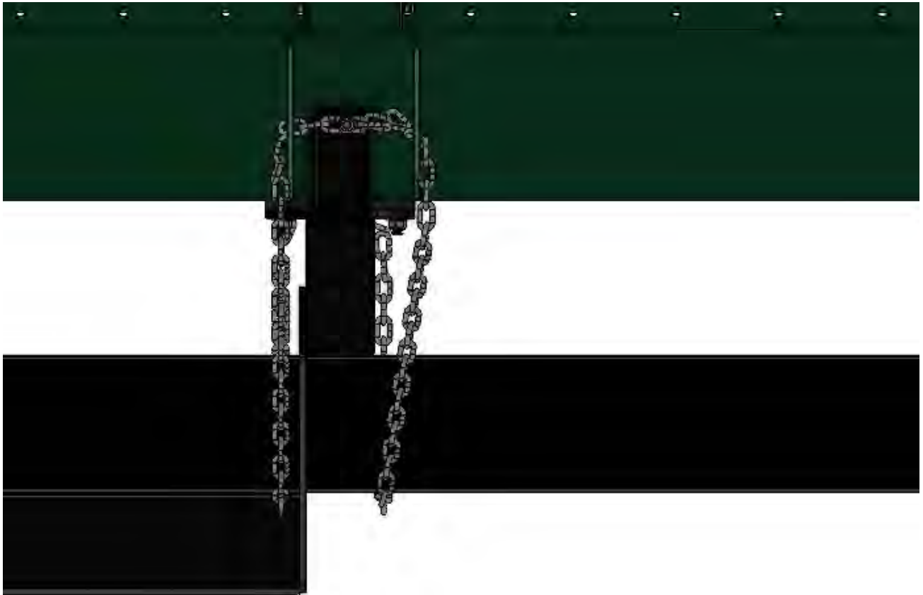
Horst 505 front lashing as seen from side of forage box.
