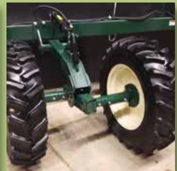
Heavy Duty Wheel Carriers Wide Walking Tandem Shown 12.4 x 24 - 8 Ply
