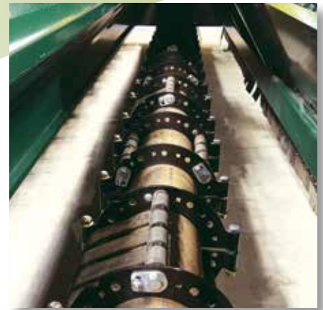
Front Rotor, Steel Cluster Cupped Knives Enclosed in shredding shroud
