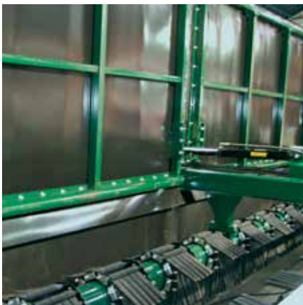
Easy Access, Heavy Duty Belted Top Covers Two belted top covers with single cylinder hydraulic open
