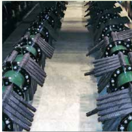
Center Rotor, 6-pin Rubber Flails Rear Rotor, 8-pin Rubber Flails
