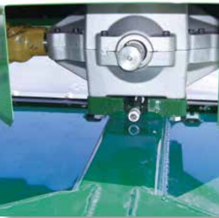
Heavy Duty Gearbox with positioned jackshaft for better PTO angle
