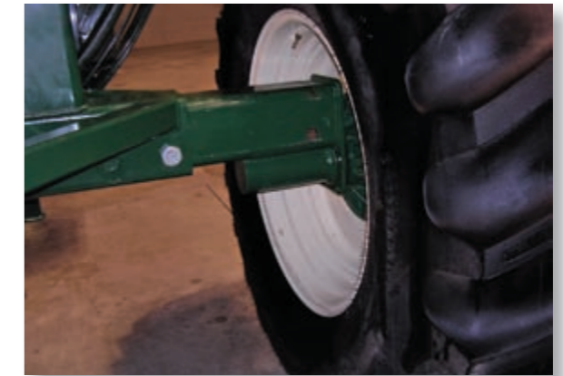
Tires and Axles — Large high flotation 24.5 x 32 or optional 30.5 x 32 - 4 1/2 in. spindles. Reduced compaction and ease of pull.
