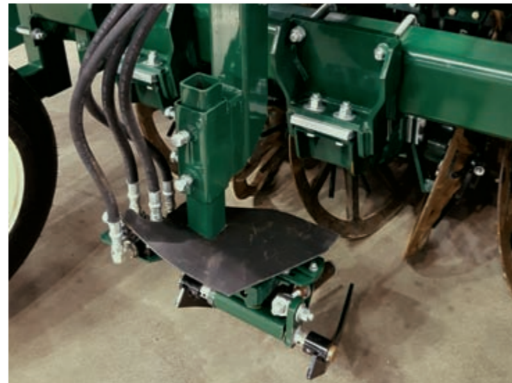
Outboard Mounted Hydraulic Row Finder provides better visibility.
