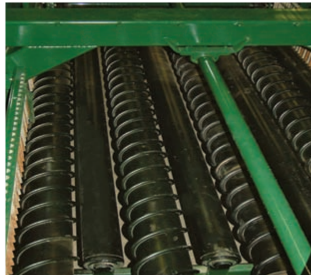
Grab Roll Bed 4 pair (8 rolls) with single point adjustment on front and rear. Individual cushions for rock protection.
