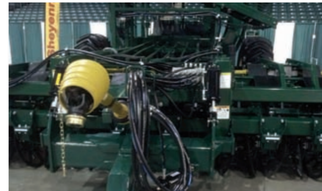
Improved hydraulic circuit. Junction blocks eliminate leak points.
