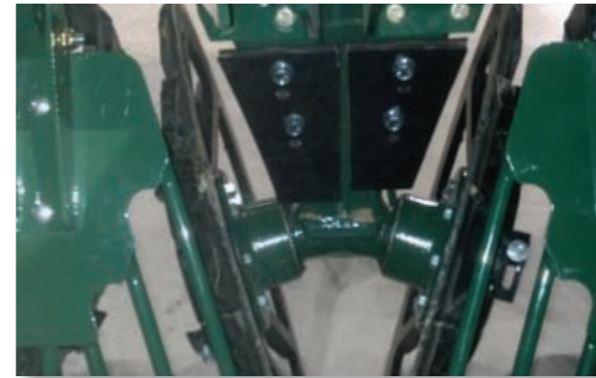
Paddle Shaft — Adjustable heavy rubber paddles and pivoting barriers keep beets in the machine.
