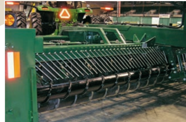
Conveyor Rolls — 4 roll conveyor with 7/8 in. diameter spiral. Fully adjustable. Dual 5 band 5V drive belt on wide heads. (Rear grab roll optional shown)
