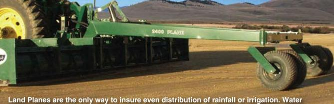
Land Planes are the only way to insure even distribution of rainfall or irrigation. Water pockets can be eliminated by utilizing the natural slope of the field. On rolling ground, landsmoothing improves surface drainage thereby controlling erosion. Tile drainage will handle sub-surface moisture, but a smooth field is necessary to remove excess surface water before damage occurs.
