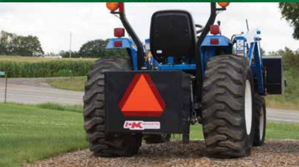
With a material holding volume of 3.5 cubic feet and maximum holding weight capacity of 525 LBS., this new weight box can add up to 575 LBS. of balancing weight to your CAT. 1 3PH. This added weight backs up your tractor by off setting your loader mounted attachments helping to keep your tractor safely balanced during operation.
