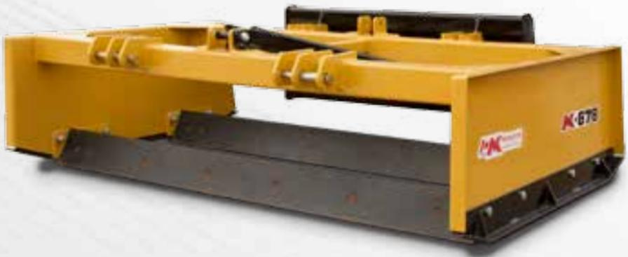
This two in one combination of leveling and scraping makes short work of your grading jobs. The first blade attacks the high spots cutting them down to size, the second blade further scrapes anything the first missed and fills in the hollows. With two blades cutting and filling it takes much less time and fewer passes to achieve the even distribution of material you are looking for.
