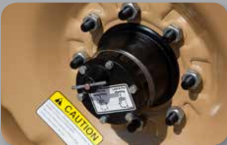
LOCK OUT HUBS - Disengages all drive components, reducing wear and tear during transport.
