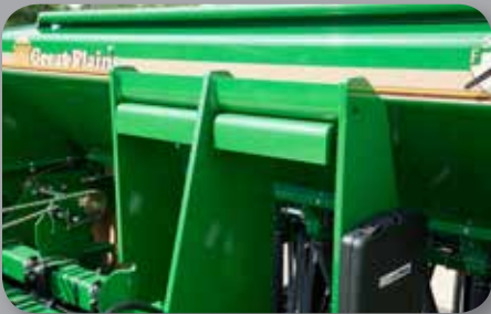
STANDARD WEIGHT BRACKETS - Add standard tractor weights to the weight brackets for even better penetration in tough no-till conditions.
