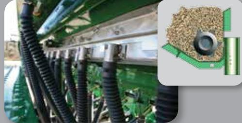
**FERTILIZER BOX** - Features stainless steel components for long life. Six-Point Star Meter Wheels accurately meter just the amount of fertilizer you desire.
