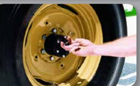
**LOCK-OUT HUBS** - Quickly disengage all chains and sprockets for reduced wear during transport.
