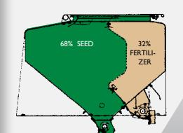
**SEED BOX CONFIGURATIONS** - The large 3.2 bushel-per-foot seed box can be split for seed and fertilizer application. In addition, an optional small seeds box that mounts directly to the back of the main seed box is available.
