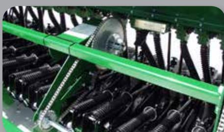
**4-SPEED SPROCKETBOX** - Provides excellent metering of a large variety of seed shapes and sizes.
