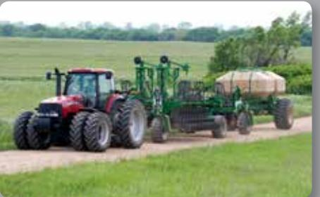
NARROW TRANSPORT - The 3N-4010HDA provides an innovative folding design that tucks nicely behind the tractor and is only slightly wider than the outside duals on most tractors.
