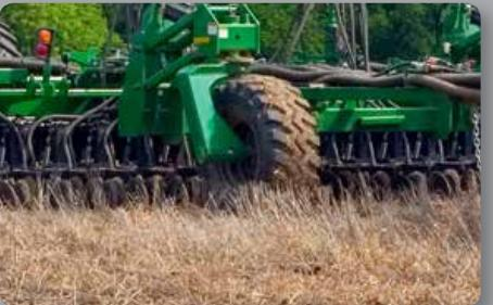
HIGH FLOTATION - The implement is carried on six (6) 18 x 22.5 tires, providing increased accuracy and reduced field compaction.
