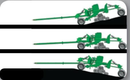
FLOATING HITCH - Provides superior terrain following because the unit covers the terrain independently of the tongue.
