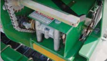
4-SPEED GEARBOX - Lifetime lubricated heavy-duty gearboxes make seed rate changes quick and effortless.
