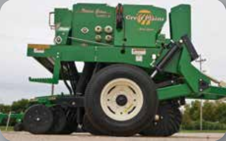
END WHEEL DESIGN - Rugged time-proven design stays on side-hills and maintains accurate seed placement in undulating terrain.
