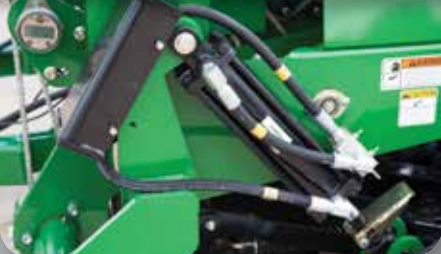
HYDRAULIC DEPTH STOP - Infinite range of adjustments to tailor coulters depth to seeding depth.
