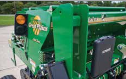
OPTIONAL WEIGHT BRACKETS - The 606NT has a weight bracket that can be added to each end of the drill to add up to 600 lbs of weight for better penetration in extremely difficult no-till conditions.
