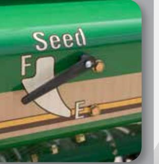
**SEED LEVEL INDICATOR** - Easy to read from the tractor seat. Our floating indicator provides an accurate reading from inside the seedbox.
