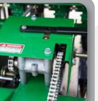
**4-SPEED GEARBOXES** - Provides increased accuracy and flexibility of the metering system by giving the operator more choices for drive speed.
