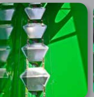
**V-BOTTOM DIVIDERS** - Allow all the seed to feed from the seedbox to the feeder cup so you get complete emptying. Dividers also help prevent seed from shifting in the box on sidehills.
