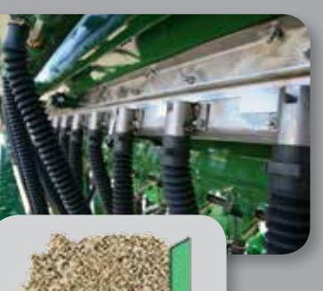
**FERTILIZER BOX** - Features stainless steel components for long life. Six Point Star Meter Wheels accurately meter just the amount of fertilizer you desire.
