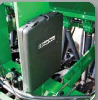
**WATERPROOF MANUAL HOLDER** - Keeps Owner and Operator Manuals flat and in good condition. Simply lift tabs to remove.
