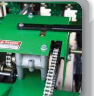
**4-SPEED GEARBOXES** - Provide increased accuracy and flexibility of the metering system by giving the operator more choices for drive speed.
