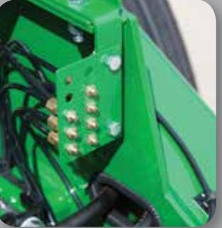
**GREASE BANK** - Installed on no-till machines so all coulters can be serviced from a centralized location.
