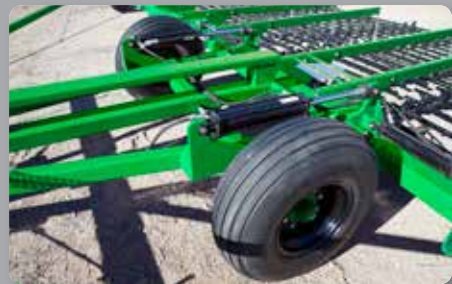
TRANSPORT TIRES – Extra heavy 8-bolt transport hubs and wheels. Six-bolt wing hubs and wheel with bolt in spindles for more tire stability and reliability.
