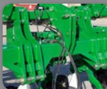
3-POINT HITCH - The 3-point lift frame extends the length of the center section, creating a fully trussed mainframe. The Lister Cultivator is available in category 3, 3N, 4, and 4W configurations.
