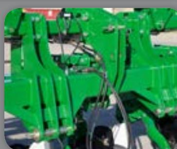
3-POINT HITCH - The 3-point lift frame extends the length of the center section, creating a fully trussed mainframe. The Lister Cultivator is available in category 3, 3N, 4, and 4W configurations.
