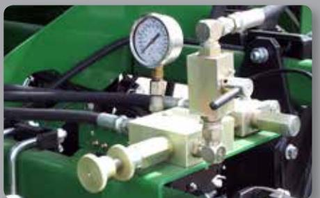
**HYDRAULIC WEIGHT TRANSFER** - Transfers weight from the center frame to the wings, allowing even distribution of weight across the entire width of the implement.
