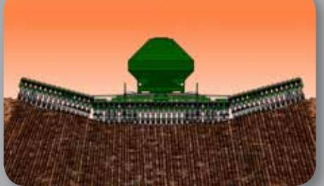
**FLEXIBILITY** - Wing flex of 15° down and 20° up for excellent ground gauging capabilities.
