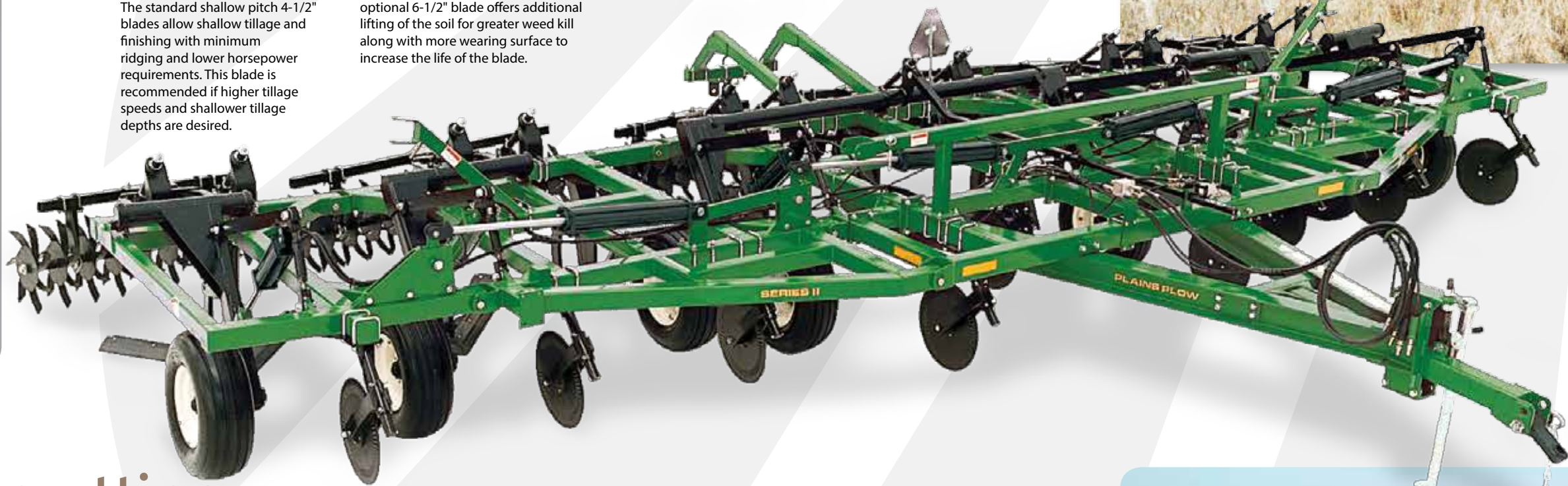
21" TREADER WHEEL - 7" spacing is ideal for breaking clods, uprooting weeds, and preparing a seedbed. Hard faced for long life.
