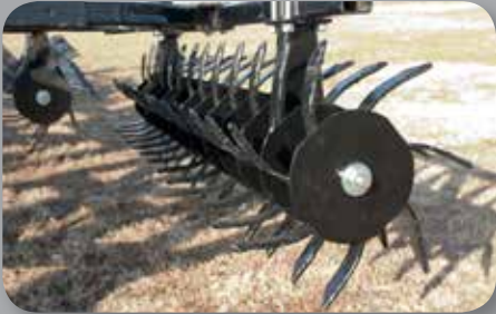
21" TREADER WHEEL - 7" spacing is ideal for breaking clods, uprooting weeds, and preparing a seedbed. Hard faced for long life.
